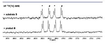
Figure 11. Fragments of high pressure  ${}^{31}P{}^{1}H$  NMR spectra of Rh(L5) complexes (0.01 M solution) in the presence of 10 equiv of substrate 5 (above) or product 8 (below) and 15 equiv of TEA, formed in situ, under 5 bar of syngas (CO/H<sub>2</sub>, 1:1) measured in CD<sub>3</sub>CN; # and \* denote signals of different phosphorus atoms.
