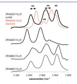
**Figure 4.** High pressure infrared (IR) spectra of  $[Rh(Ln)(CO)_2H]$  complexes (0.001–0.002 M solutions) for phosphine ligands L1–L4, formed in situ, under 20 bar of syngas (CO/H<sub>2</sub>, 1:1; alternatively CO/D<sub>2</sub>, 1:1 for the deuterated species–spectrum in red) measured in CH<sub>2</sub>Cl<sub>2</sub>.
