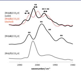
**Figure 6.** High pressure infrared (IR) spectra of  $[Rh(Ln)(CO)_2H]$  complexes (0.001–0.002 M solutions) for phosphite ligands L5–L7, formed in situ, under 20 bar of syngas (CO/H<sub>2</sub>, 1:1; alternatively CO/D<sub>2</sub>, 1:1 for the deuterated species–spectrum in red) measured in CH<sub>2</sub>Cl<sub>2</sub>; the assignment of the signals was verified with DFT calculations.
