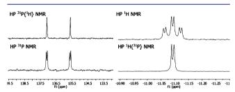
Figure 7. High pressure (HP) NMR spectra of  $[Rh(L6)(CO)_2H]$  complex (0.014 M solution), formed in situ, under 5 bar of syngas  $(CO/H_2, 1:1)$  measured in  $CD_2Cl_2$ .
