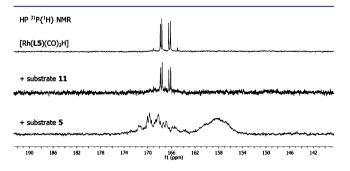
**Figure 10.** High pressure <sup>31</sup>P{<sup>1</sup>H} NMR spectra of Rh(LS) complexes (0.01 M solution) in the absence (above) and in the presence of 10 equiv of substrate **11** (middle) or substrate **5** (below) and 15 equiv of TEA, formed in situ, under 5 bar of syngas (CO/H<sub>2</sub>, 1:1) measured in CD<sub>3</sub>CN + CD<sub>2</sub>Cl<sub>2</sub> (1:1).
