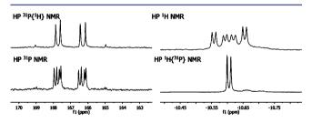
Figure 5. High pressure (HP) NMR spectra of  $[Rh(L5)(CO)_2H]$  complex (0.02 M solution), formed in situ, under 5 bar of syngas  $(CO/H_2, 1:1)$  measured in  $CD_3CN + CD_2Cl_2$  (1:1).
